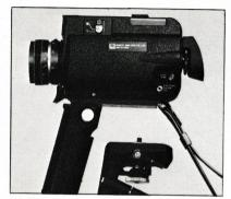
• Fit a tripod into the hole in the bottom of the camera body.
